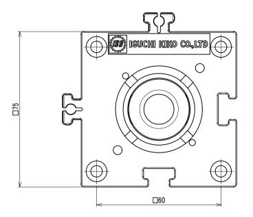
Details: Ball transfer unit: IP-16 Insert Method:Insert from bottom of puzzle unit (as shown in drawing)
